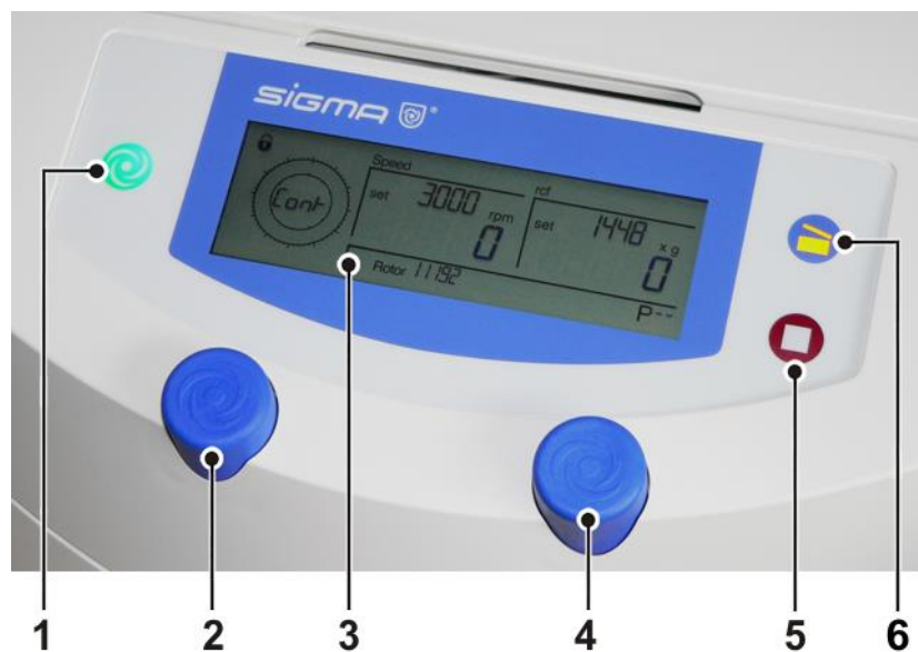
Fig. 8: User interface of the "Spincontrol Universal" control system
