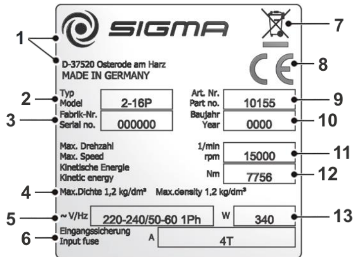
Fig. 3: Example of a name plate
