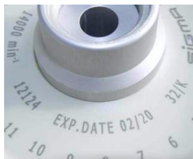
Fig. 4: Different service life – engraving on the bucket/rotor
