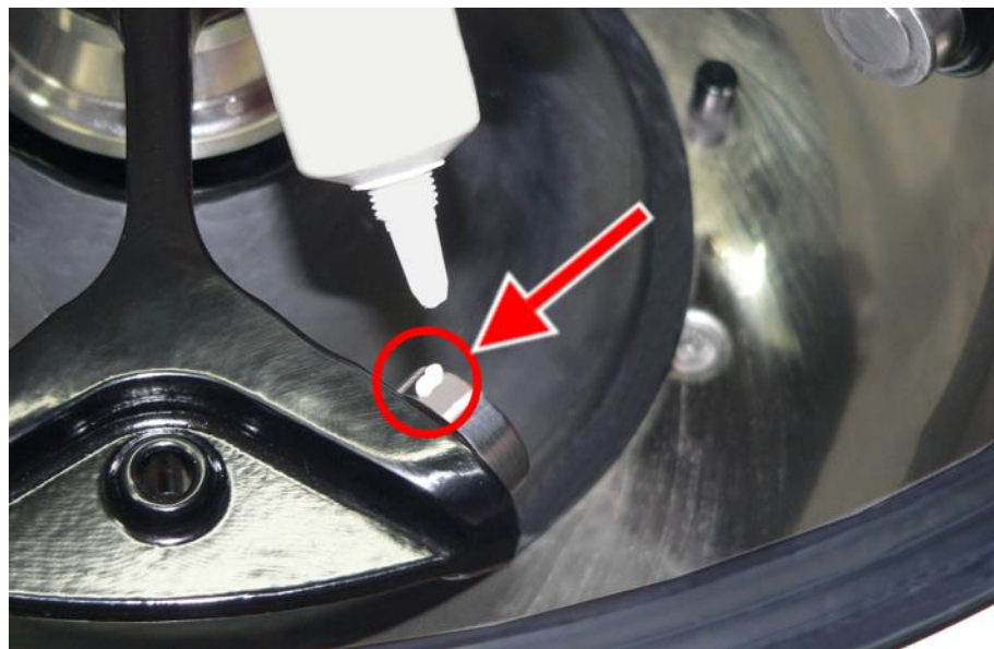
Fig. 21: Sufficient quantity of grease for one bolt
