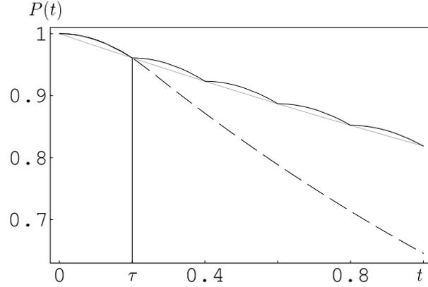
Fig. 4: Quantum Zeno effect for  $N = 5$  “pulsed” Von Neumann measurements. The dashed (full) line is the survival probability without (with) measurements. The gray line is the interpolating exponential (3.18). As  $N$  increases,  $p^{(N)}(t) \rightarrow 1$  uniformly in  $[0, t]$ . The units on the abscissae are arbitrarily chosen for illustrative purposes.
