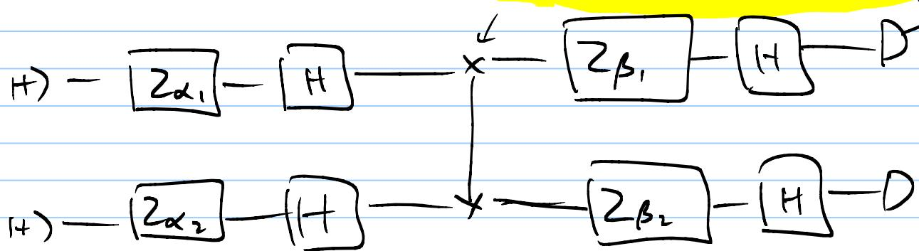
Note Pauli errors passing through a CZ gate, fan out in a light cone
