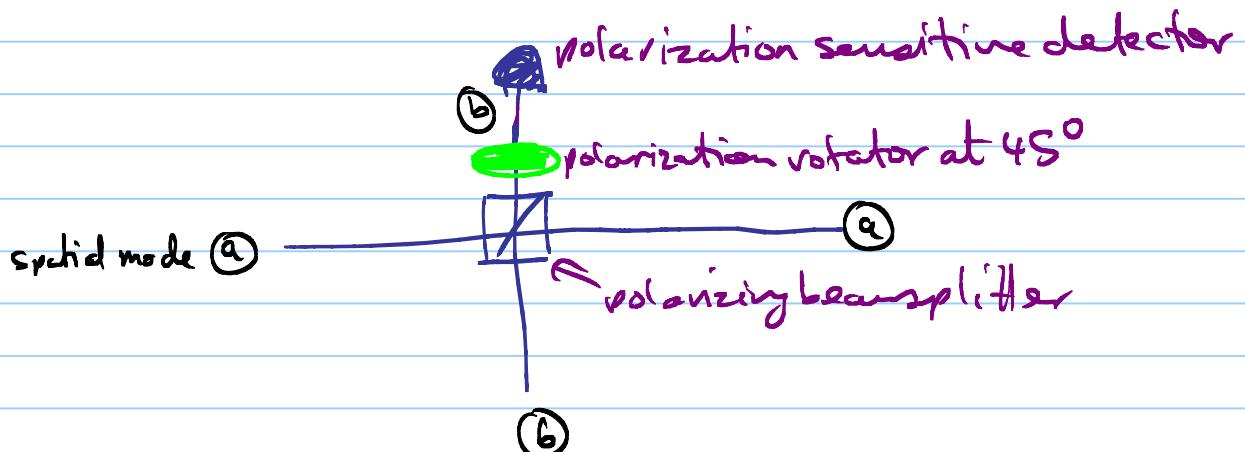
Work out the effect of the gate on four possible input pairs:
